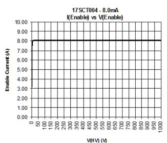
*b)* Over-Temperature protection: The current is temperature limited according to the typical curve below. This patent-pending characteristic ensures that the 17SCT004A will stay within a reasonable temperature range (<~150C) under normal operation. This is particularly true when high-current ranges of 15 or 21mA
