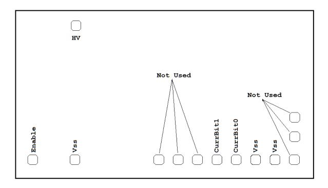
"Not Used" Pads should be left open and should not be connected to Vss or to one another.
