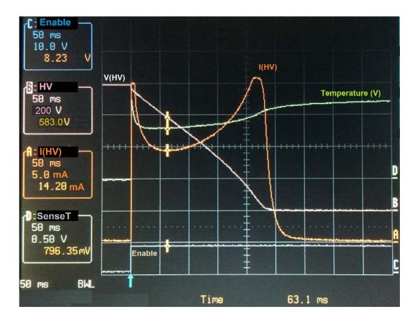
The discharge shown by trace B (HV) is essentially completed in 250-300mSec at a maximum current of ~25mA. For this example we purposely programed this chip to 25mA, somewhat above the specified maximum 21mA specification.
