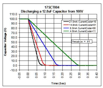
In this example the capacitor's energy is relatively small (~65mJ) and self-heating is below the threshold for over-temperature protection to be in effect.
